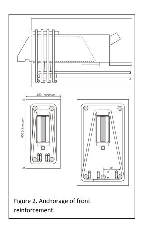
As illustrated in the left section in figure 2 it will be congested if the beam has minimum dimensions. This must be taken into account when the anchorage length of the horizontal U-shaped bars is calculated. (The main reinforcement of the beam is not shown in the side view.)
