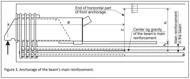
The force is approximately  $[F_V \times \frac{a}{z} + \frac{F_V}{2} + F_H \frac{x_1}{z}]$ . Additional force in the beam's top reinforcement is about
