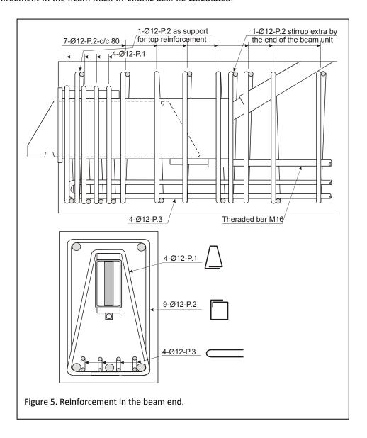
At the end of the horizontal part of the front anchorage (P.3) it must be checked that the beam's main reinforcement has sufficient anchorage. See clause 2.2.2.
