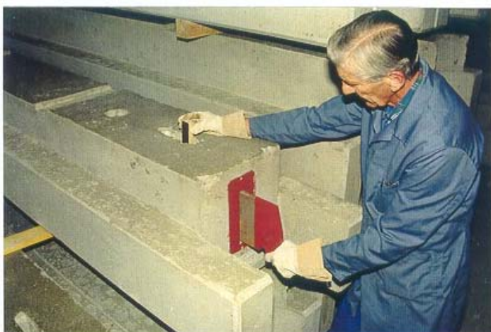
4.45 The BSF-knife is easy to move.
