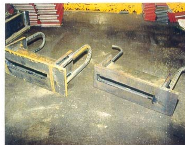
2.12 Eksample of reinforcement welded on to one-sided column units
