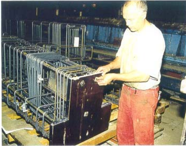
3.31 BF-unit fastened through spaced holes in end plate with screws.
