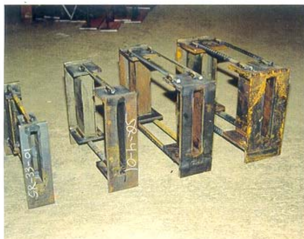
2.11 Double column units after welding.
