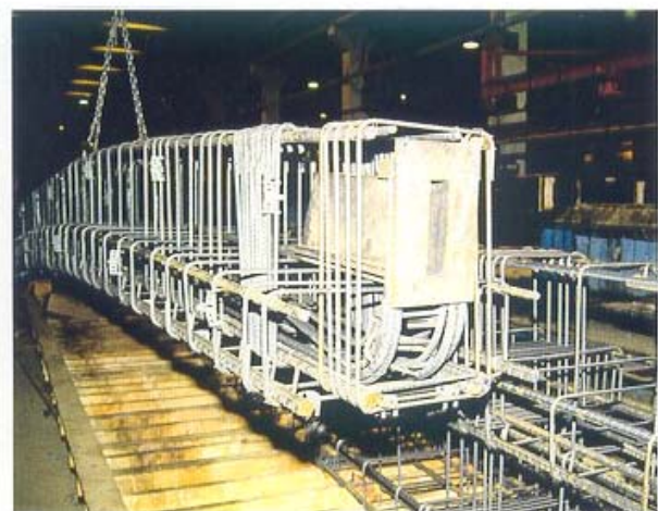
3.28 BF 200/40 placed in reinforcement.
