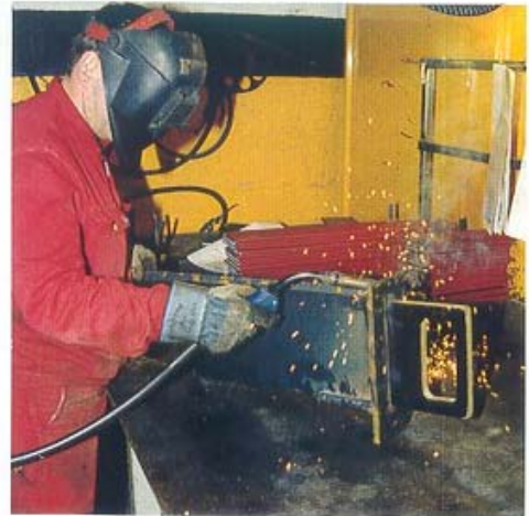
3.26 BF 200/20 upside/down, reinf. spot welded. Plywood plate for correct position.
