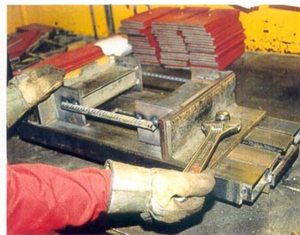
2.10 The jig is adjustable.
