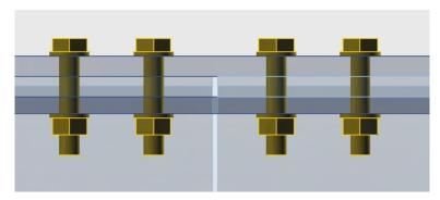
In the connection with more shear sections is shear force in bolt divided into appropriate number of sections. Values in all shear sections are printed in the table (divided by slash). The check is done for each section separately.
