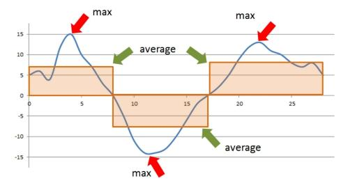
Version 5.3 has improved averaging for thin walled cross-section with arcs. Welds on all parts of the cross-section are considered as one weld. Parts with the same sign are determined on this weld. Results are much more realistic.
