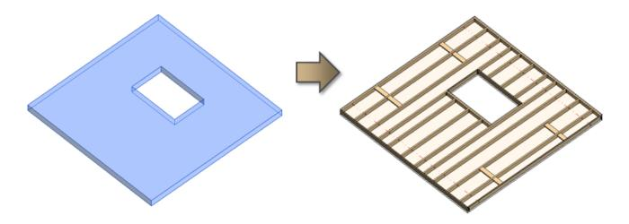
Note: frame direction depends on the Span Direction in the Floor Boundary:
