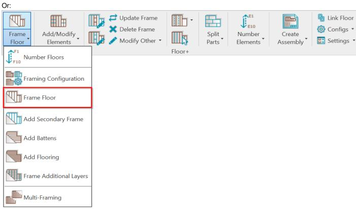
Frame Floor – frames selected floors or parts from the model according to predefined configuration.
