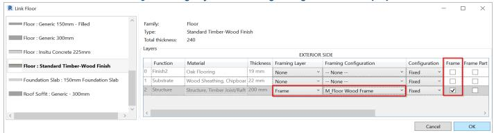
There is no problem if framing configuration in not assigned to the layer. You can assign it in the **Link Floor** dialog, or **Floor+** will give you this option during the **Frame Floor** process:
