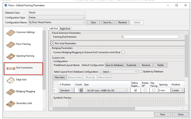
Floor+ supports various types of end connections. End connection joists are parallel to floor direction line.
