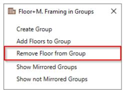
**Remove Floor from Group** – removes floor together with frame from selected group. Usually used before making modifications to frame.
