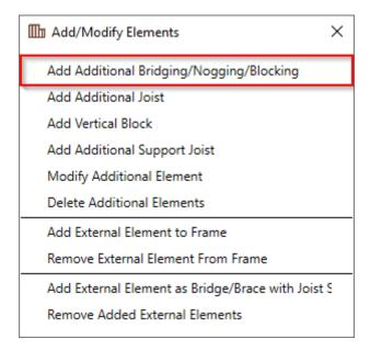
**Add Additional Bridging/Nogging/Blocking** – adds additional bridging/nogging/blocking between two selected joists with predefined settings.
