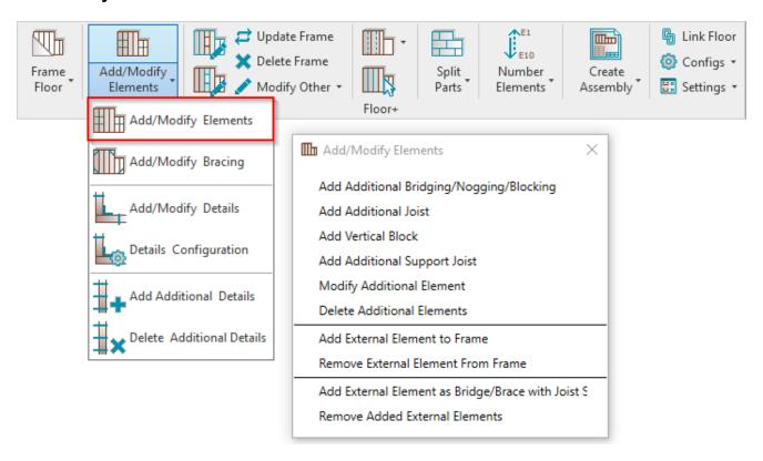
Add/Modify Elements – features for adding/modifying additional joists, support joists, bridging/nogging elements, etc.
