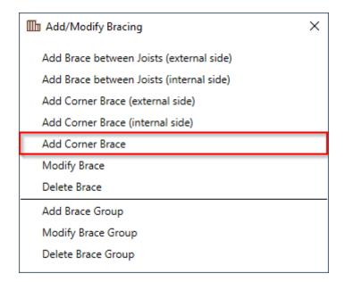
Add Corner Brace – adds a corner brace between a rim joist and a joist. To modify brace settings go to Floor+ → Add/Modify Elements → Add/Modify Bracing → Modify Brace.
