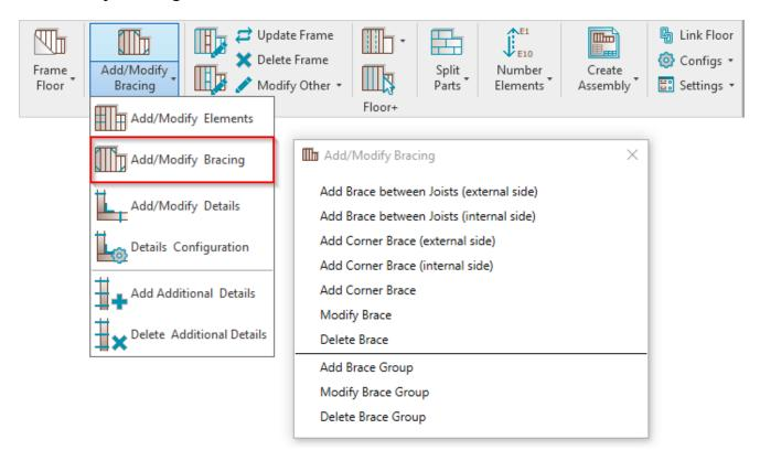
**Add/Modify Bracing** – features for adding/modifying braces between joists or rim joists, corner braces and brace groups.
