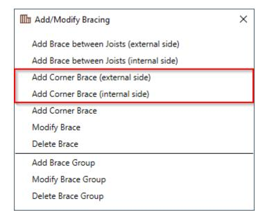
Add Corner Brace (external/internal side) – adds a corner brace between a selected rim joist and joist on external or internal side of framing. To modify brace settings go to Floor+ → Add/Modify Elements → Add/Modify Bracing → Modify Brace.
