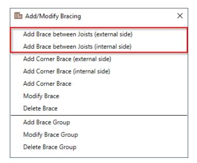
Add Bracing between Joists (external/internal side) – adds a brace between two selected joists on external or internal side of framing. To modify brace settings go to Floor+  $\rightarrow$  Add/Modify Elements  $\rightarrow$  Add/Modify Bracing  $\rightarrow$  Modify Brace.
