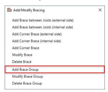
Add Brace Group – places short braces automatically between two joists with predefined rules.
