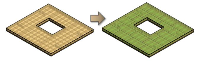
Sheathing or Paneling will be split if selected floor layer has the conditions below in Link Floor:
