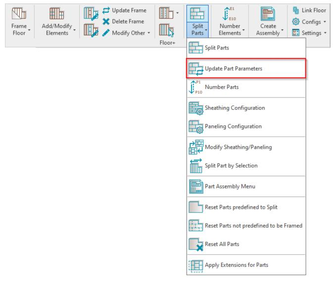
Update Part Parameters – updates part parameters from Sheathing/Paneling Configuration → Mark Settings without needing to use Split Parts on the floor again. Also enters HostMemberSortMark parameter.
