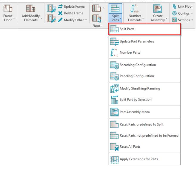
**Split Parts** – splits sheathing or paneling into segments by predefined **Sheathing Configuration** or **Paneling Configuration**. You just need to select a floor or any frame of a floor.
