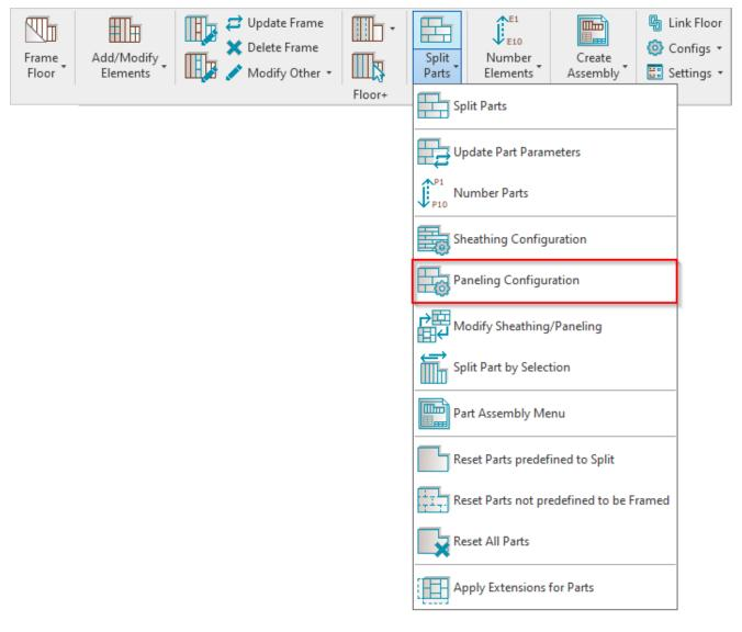
**Paneling Configuration** – allows you to configure and save settings for the paneling layouts. These settings can be saved and linked with floor layer using **Link Floor**.
