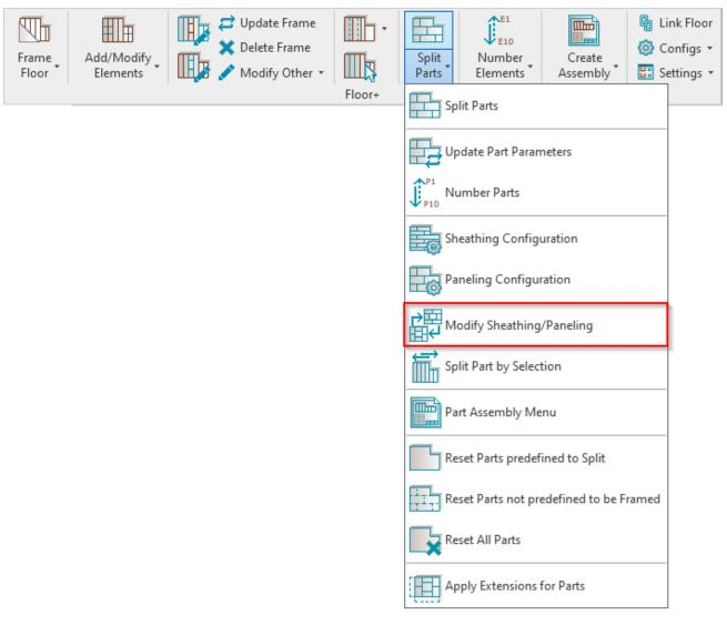
**Modify Sheathing/Paneling** – changes selected floor layer sheathing/paneling configuration to the new one from the list.
