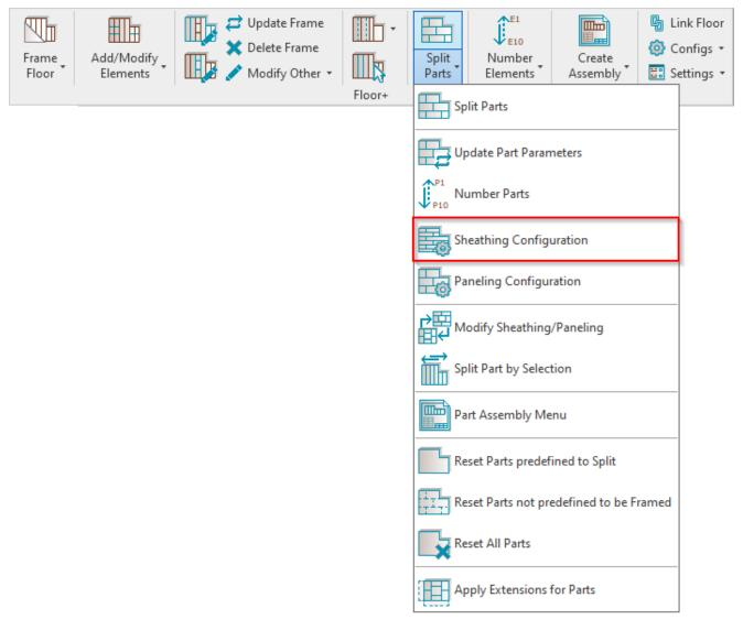
**Sheathing Configuration** – allows you to configure and save settings for the sheathing layouts. These settings can be saved and linked with floor layer using **Link Floor**.
