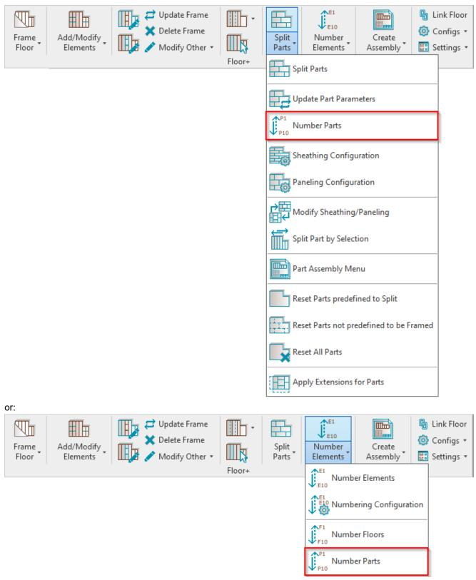
Number Parts – renumbers all sheathing/paneling elements (Parts) by predefined configuration in Numbering Setup → Part Numbering Configuration. Part numbering configurations come from Sort Mark (http://www.aga-cad.com/products/tools4revit/sort-mark).
