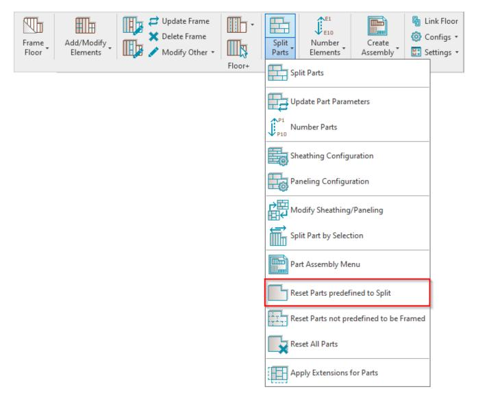
Reset Parts predefined to Split - resets sheathing/paneling layout to a single part.
