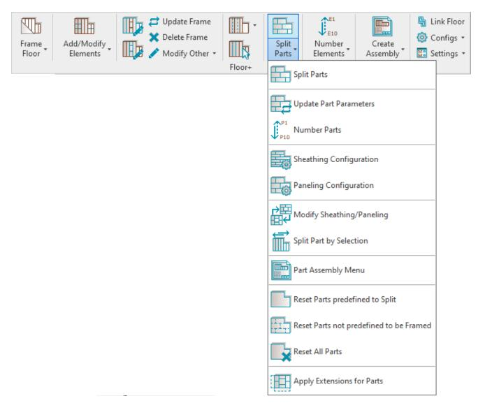
**Wood Framing Floor+** automates the creation of sheathing and paneling layouts. Sheathing or paneling layouts can be generated and split by existing joists or other predefined rules.
