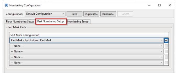
Example: All sheathing/paneling elements (Parts) are grouped by **Framing Member Mark**, uniquely numbered, and have **Framing Member Mark** value as a prefix. Result is written to the **Mark** instance parameter.
