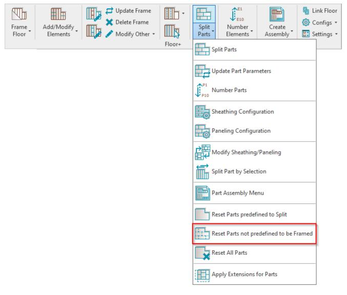
Reset Parts not predefined to be Framed – resets sheathing/paneling parts that were not predefined to be framed.
