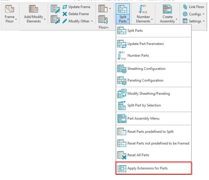
**Apply Extensions for Parts** – applies extensions for sheathing/paneling parts and merges all part segments. Extension values come from **Sheathing** or **Paneling Configuration**.
