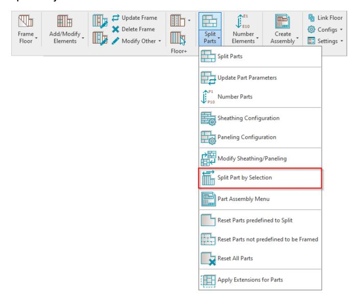
**Split Part by Selection** – splits selected sheathing/paneling layout by predefined placement direction: **From Start**, **From End**, or **From both Sides**.
