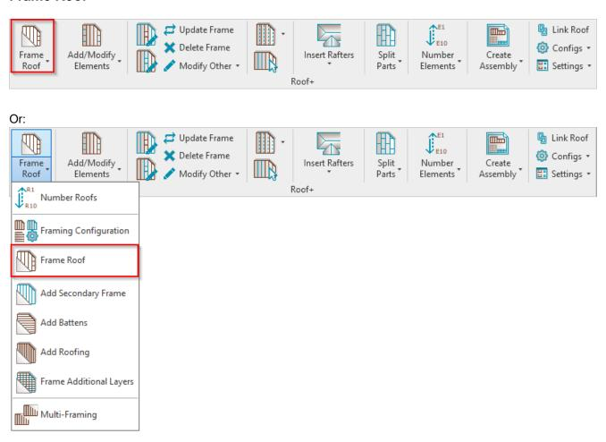
Frame Roof – frames selected roofs or parts from the model according to predefined configuration.
