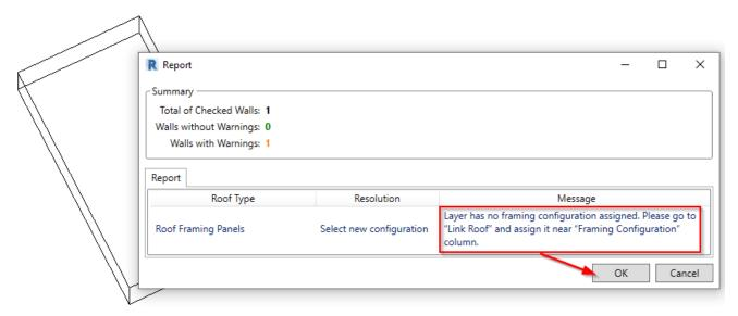
Selected a sample framing configuration, which automatically comes with Roof+, and click OK:
