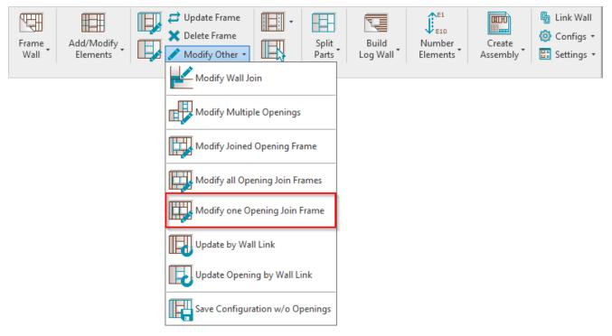
**Modify one Opening Join Frame** – modifies a single window, door, or other joined opening common framing, like trimmers or cripples, by custom settings if you need to make unique changes. All configuration settings are the same as in Framing Configuration.
