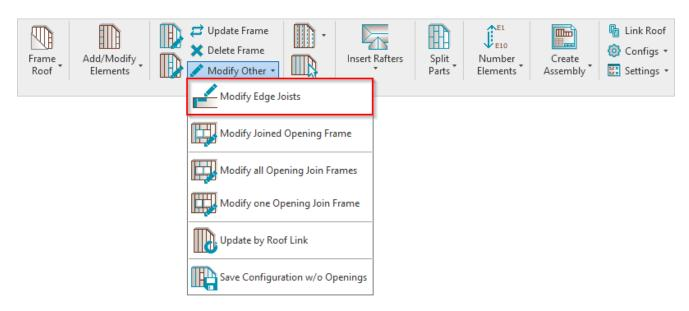
**Modify Edge Joins** – modifies selected join by custom settings if you need to make unique changes. All configuration settings are the same as in **Framing Configuration**.
