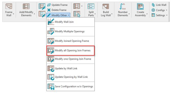
**Modify all Opening Join Frames** – modifies selected joined window, door, or other opening common framing, like trimmers and cripples, by custom settings if you need to make unique changes. All configuration settings are the same as in **Framing Configuration**.
