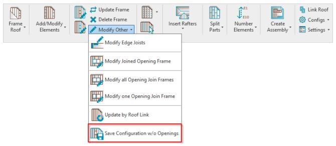
**Save Configuration w/o Openings** – saves configuration of selected frame without settings for openings. This feature is very useful if you have already framed a roof and you lost the configuration that was used for it. The configuration is needed to frame new roofs.
