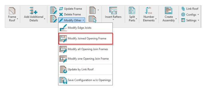
**Modify Joined Opening Frame** – modifies selected joined window, or other opening framing by custom settings if you need to make unique changes. All configuration settings are the same as in **Framing Configuration**.
