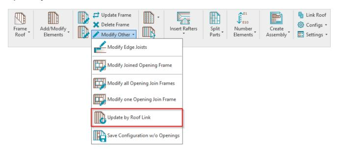
Update by Roof Link – reframes selected roof frame to default, which is configured under Framing Configuration.
