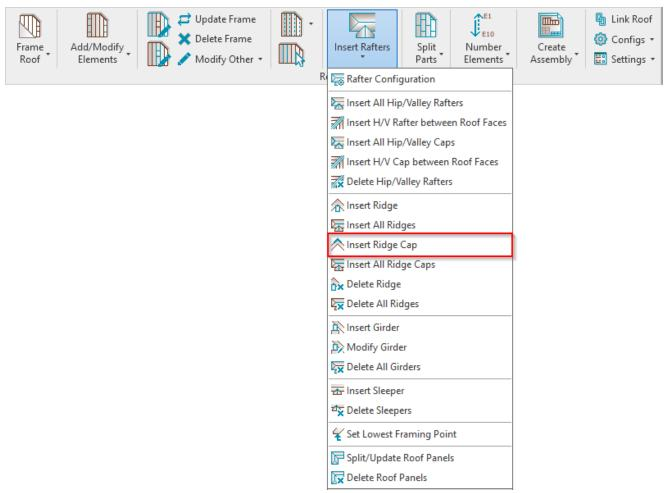
**Insert Ridge Cap –** inserts ridge cap on selected roof panel. Before inserting, predefine ridge cap type in **Rafter Configuration**.
