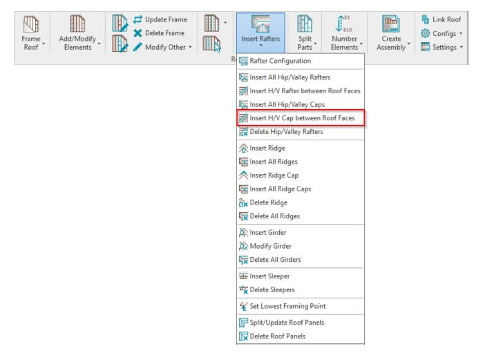
**Insert H/V Cap between Roof Faces** – inserts hip or valley caps between two selected roof faces. Before inserting, predefine hip and valley cap types in **Rafter Configuration**.
