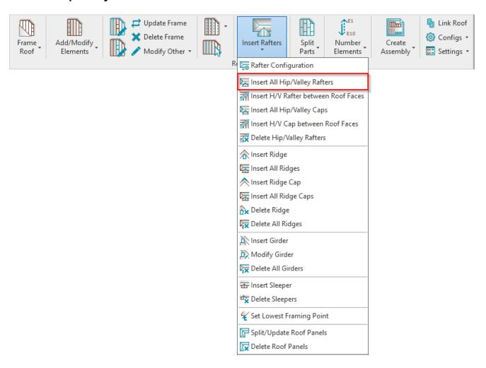
**Insert all Hip/Valley Rafters –** inserts hip and valley rafters in selected roof. Before inserting, predefine hip and valley rafter types in **Rafter Configuration**.
