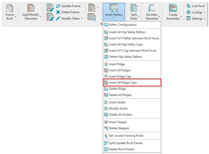
**Insert all Ridge Caps** – inserts all ridge caps on selected roof. Before inserting, predefine ridge cap type in **Rafter Configuration**.
