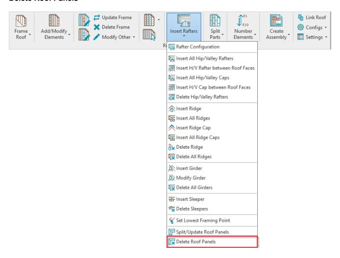
**Delete Roof Panels –** deletes all roof panels from selected roof.
