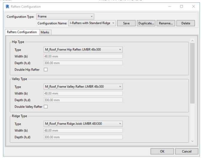
**Rafter Configuration –** defines hip, valley, ridge, girder, and sleeper settings. These settings can be saved under different names and for different roofs.
