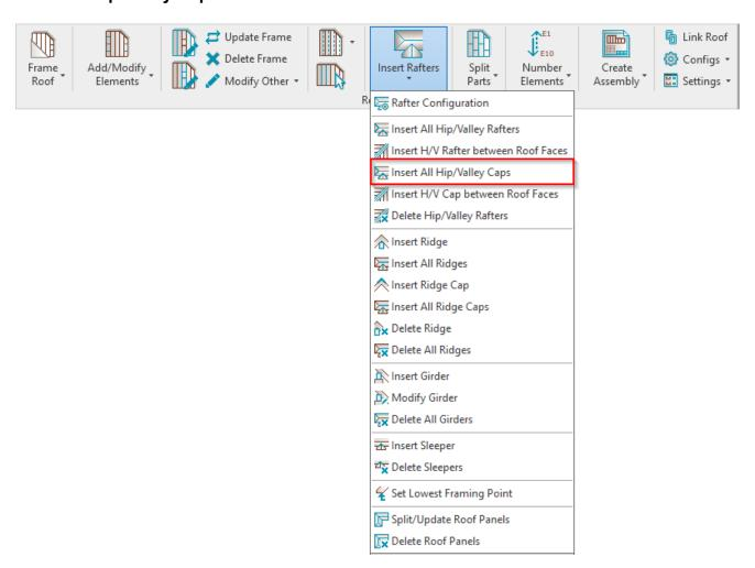
**Insert all Hip/Valley Caps –** inserts hip and valley caps on selected roof. Before inserting, predefine hip and valley cap types in **Rafter Configuration**.
