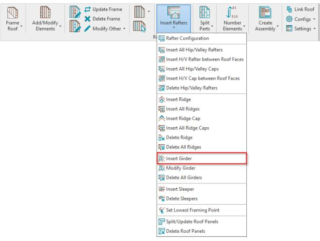
Insert Girder - inserts girder beam between two selected hip, valley, or common rafters.
