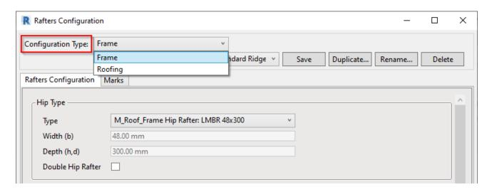
**Configuration Type** – all settings are grouped separately for the main frame and for the roofing.
