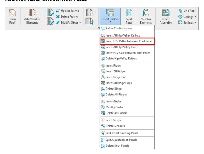
**Insert H/V Rafter between Roof Faces –** inserts hip or valley rafters between two selected roof faces. Before inserting, predefine hip and valley rafter types in **Rafter Configuration**.
