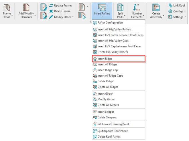
**Insert Ridge –** inserts ridge beam in selected roof panel. Before inserting, predefine ridge type in **Rafter Configuration**.
