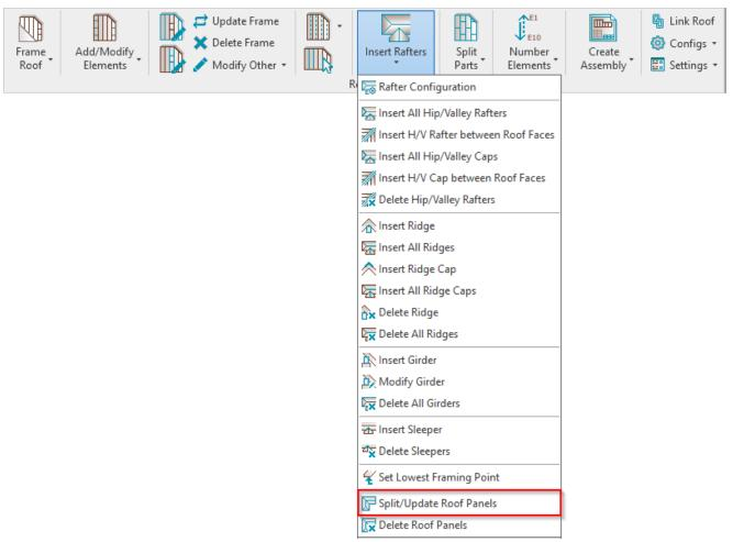
**Split/Update Roof Panels** – splits or updates panels for selected roof. Every roof slope will be recreated as a separate roof segment for proper roof framing.
