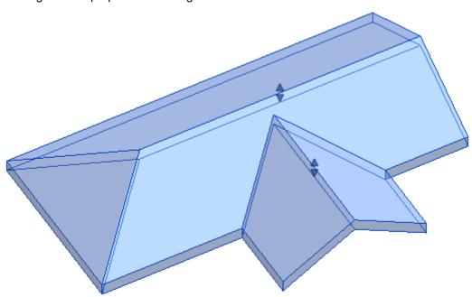
Result: Selected single roof is split into separate roof segments.
