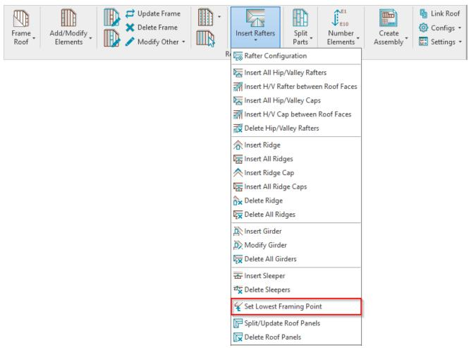
**Set Lowest Framing Point –** reads **Delta\_Z** instance parameter value from selected joist and, after clicking **Update Frame**, this value is changed accordingly for the other joists of the selected frame. Selected joist's **Delta\_Z** parameter becomes 0.
