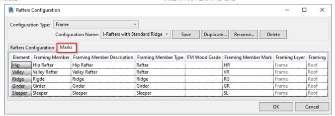
**Marks** – naming convention of framing members. You can set individual mark settings for each part of the frame for easy preparation of shop drawings. The column names are shared parameters that will be used later in schedules and tags.
