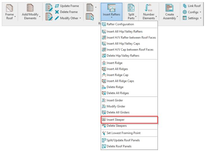
**Insert Sleeper** – inserts sleeper on selected roof face. Before inserting, predefine sleeper type in **Rafter Configuration**.
