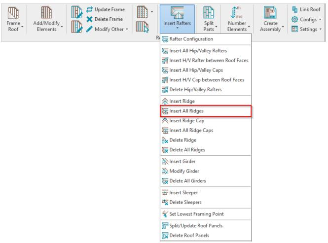
Insert all Ridges – inserts all ridges in selected roof. Before inserting, predefine ridge type in Rafter Configuration.
