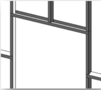
C+U Special window header (3D view):
