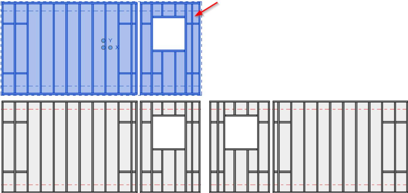
*Now wall with frame is removed from the group. You can modify it using **Modify Frame**, or other modification features:*
