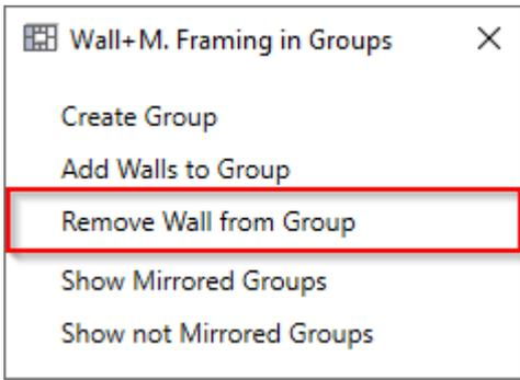
**Remove Wall from Group** – removes wall together with frame from selected group. Usually used before making modifications to frame.
