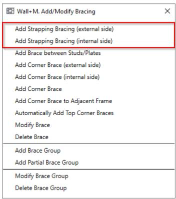
Add Strapping Bracing (external/internal side) - adds straps between two selected studs or plates.
