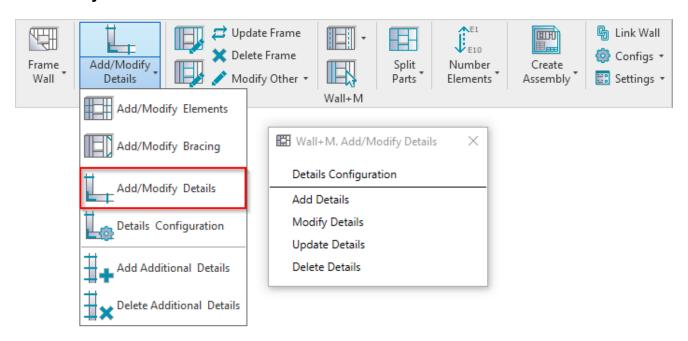
**Add/Modify Details** – for placing details in the frame. It is recommended to use these functions at the end of the framing process.
