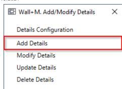
**Add Details** – adds details into selected walls according to predefined configuration. Recommended to use this function at the end of the framing process.
