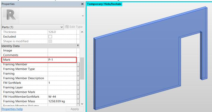
This value will be used as the assembly name. You can find shop drawings in **Project Browser** under **Assemblies**. An assembly combines all parts in a single entity, which is scheduled and isolated to create shop drawing views with tags and dimensions.
