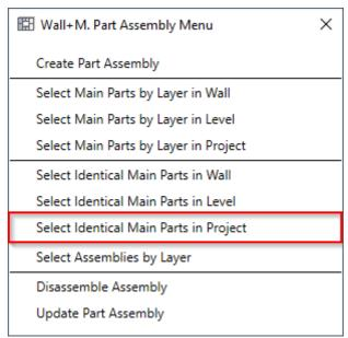
**Select Identical Main Parts in Project –** selects identical main parts of framed walls in the whole project.
