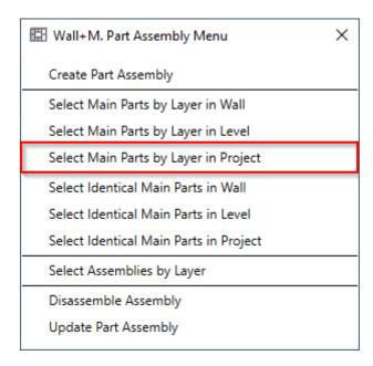
Select Main Parts by Layer in Project - selects main parts in wall frames of the same type in the whole project.
