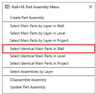
Select Identical Main Parts in Wall - selects identical main parts in the framed wall.
