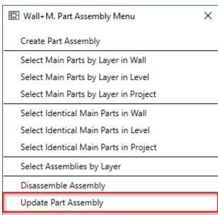
**Update Part Assembly –** updates the selected part assembly if any changes were made to the parts or to the **Drawing Configuration**.
