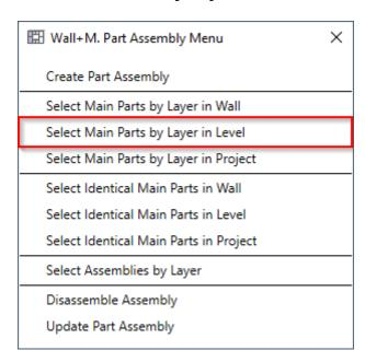
Select Main Parts by Layer in Level - selects main parts in wall frames of the same type in the same level.
