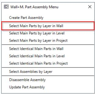
Select Main Parts by Layer in Wall – selects main parts in the framed wall.
