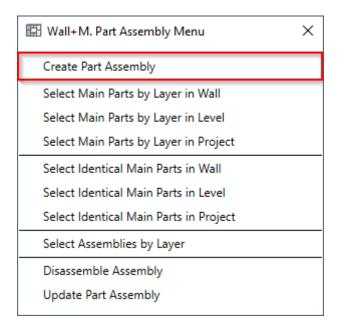
**Create Part Assembly** – makes shop drawings for selected framed parts. Select any frame of the wall and click Create Part Assembly. The software will create shop drawings according to predefined configurations. You can find shop drawings in Project Browser under Assemblies.
