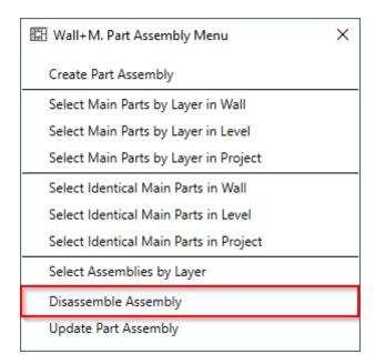
**Disassemble Assembly** – removes the assembly relationship between elements in the selected assembly and all associated views.
