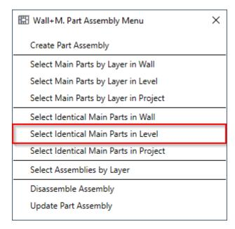
Select Identical Main Parts in Level - selects identical main parts of framed walls in the same level.
