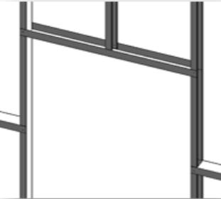
C+U Special warren diagonal cripples above the window (Front side view):
