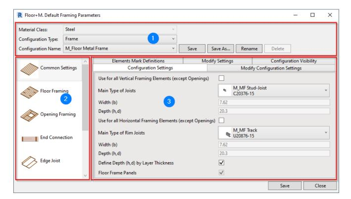
The **Framing Configuration** dialog is divided into three main parts: **Top (1)**, **Left (2)**, and **Right (3)**. In the Top part, choose the **Configuration Type** that you want to use and **Configuration Name** that you want to modify
