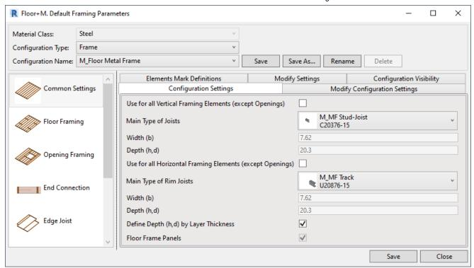
**Framing Configuration** – defines all framing settings. It allows user to configure and save settings for all sorts of frames – **Main Floor Frame**, **Secondary Frames**, **Battens**, **Flooring**. It is very a versatile tool with thousands of possibilities.
