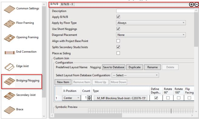
You can add different types of continuous or non-continuous **Bridging**, **Nogging** or **Blocking** into framing using different rules.
