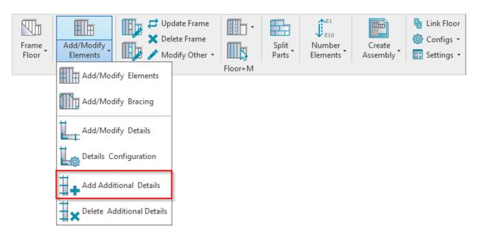
Add Additional Details – adds additional details by predefined rules to selected joist or rim joist.
