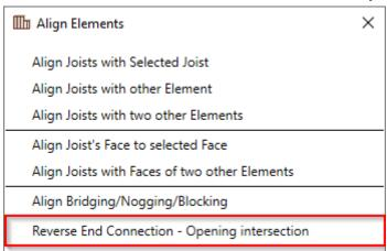
**Reverse End Connection - Opening Intersection** – used when opening is located in the frame end. Usually king stud stays and end stud is removed. While using this function end stud stays and openings' horizontal elements connect to end stud.
