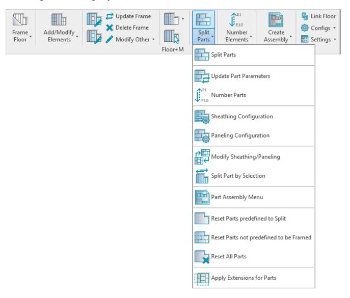
**Metal Framing Floor+** automates the creation of sheathing and paneling layouts. Sheathing or paneling layouts can be generated and split by existing joists or other predefined rules.
