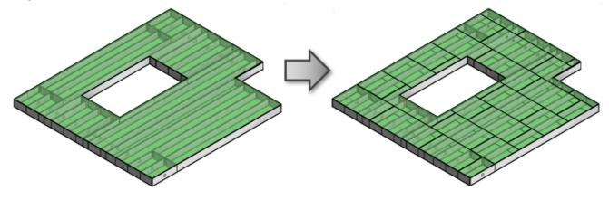
Sheathing or Paneling will be split if selected floor layer has the conditions below in Link Floor:
