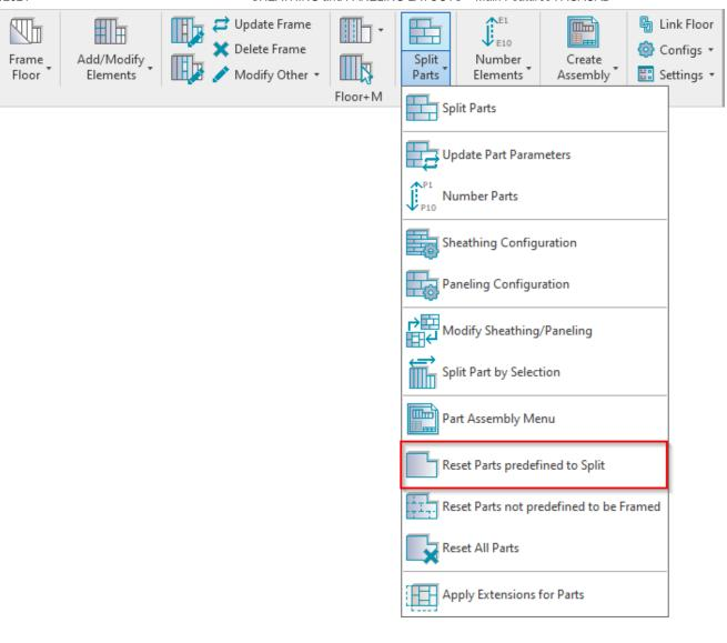
Reset Parts predefined to Split – resets sheathing/paneling layout to a single part.
