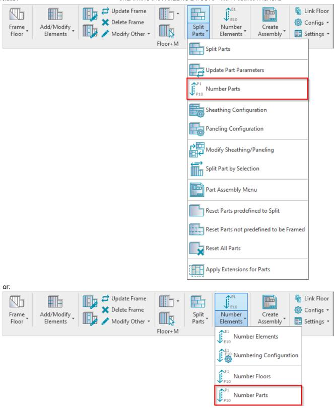
Number Parts – renumbers all sheathing/paneling elements (Parts) by predefined configuration in Numbering Setup → Part Numbering Configuration. Part numbering configurations come from <u>Sort Mark (http://www.aga-cad.com/products/tools4revit/sort-mark)</u>.
