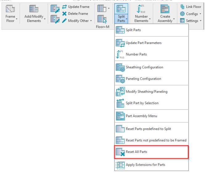
**Reset All Parts** – resets all sheathing/paneling layouts from selected floor.
