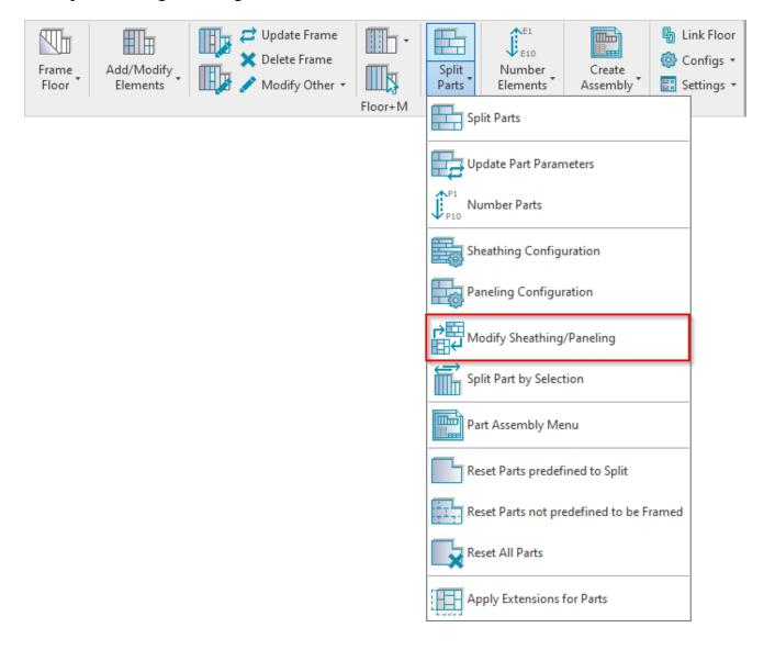
**Modify Sheathing/Paneling** – changes selected floor layer sheathing/paneling configuration to the new one from the list.
