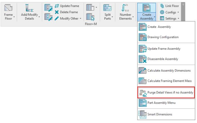
Purge Detail Views if no Assembly - removes detail views if assembly has been disassembled.
