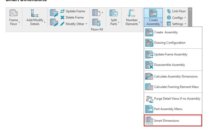
**Smart Dimensions –** features for setting up dimensions in shop drawings.
