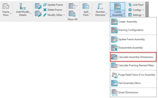
Calculate Assembly Dimensions – calculates assembly dimensions (area, volume, width, depth, length, height) by predefined rules and writes the results in assembly instance parameters (Assembly Area, Assembly Volume, Assembly Width, Assembly Depth, Assembly Length, Assembly Height) for later use in schedules.
