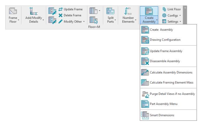
**Floor+M** will collect all elements from one floor panel and make an assembly with predefined views, add dimensions, add tags, make sheets, and put the views into the sheets.
