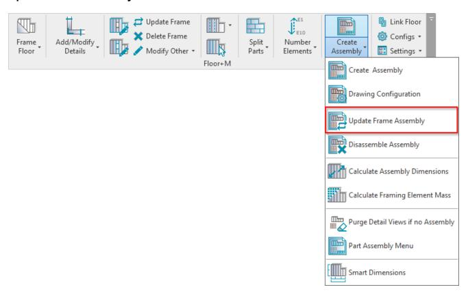
**Update Frame Assembly –** updates the selected assembly if any changes were made to the framing or to the **Drawing Configuration**.
