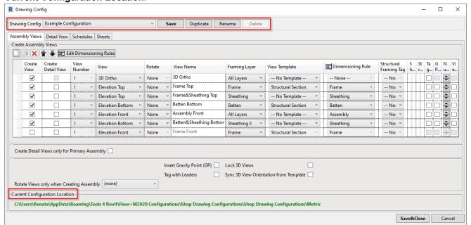
The 4 tabs (**Assembly Views**, **Detail View**, **Schedules** and **Sheets**) are for setting up assembly views, detail views, schedules, and sheets, respectively:
