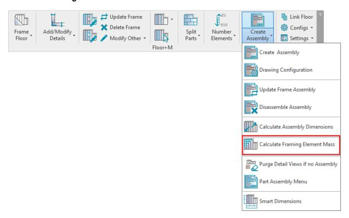
Calculate Framing Element Mass – calculates mass of selected framing elements, and writes result to Framing Member Mass parameter, which you can find in Element Properties → Identity Data.
