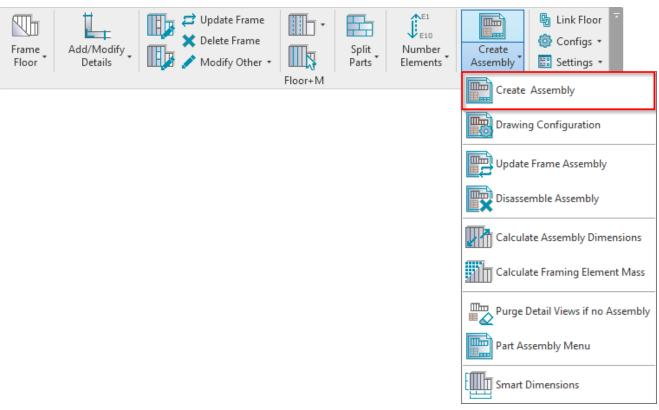
**Create Assembly** – makes shop drawings for selected floors. Select any frame from the floor, and after clicking **Create Assembly**, the software will create shop drawings according to the predefined configuration.
