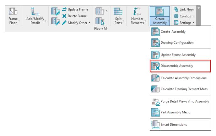
**Disassemble Assembly –** removes the assembly relationship between elements in the selected assembly and all associated views.
