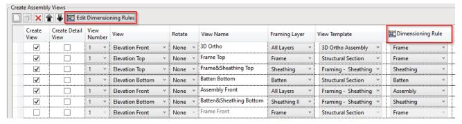
**Dimensioning Rule** – dimensioning rules for the selected view. Dimensioning rules are saved under separate names and can be used for other projects.
