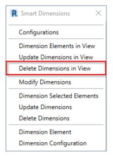
Delete Dimensions in View – deletes all dimensions that were added with Smart Dimensions from the current view.
