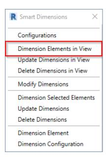
**Dimension Elements in View** – inserts dimensions for elements in the current view according to predefined configurations.
