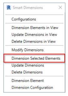
**Dimension Selected Elements –** inserts dimensions for the selected elements in the current view according to predefined configurations.
