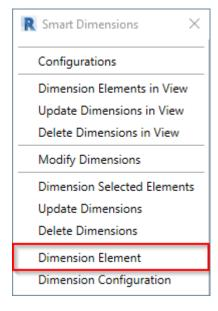
**Dimension Element –** inserts dimensions for only the selected element in the view according to **Dimension Configuration** settings.
