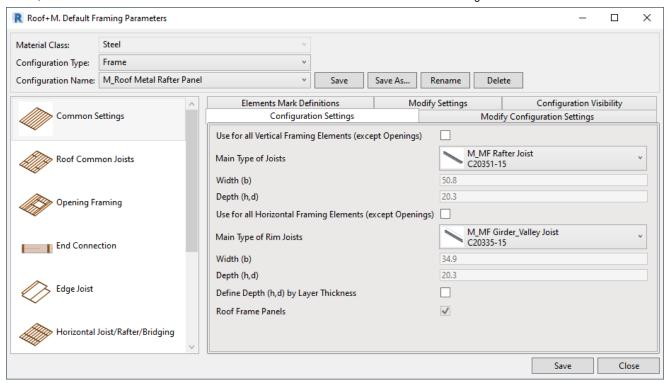
**Framing Configuration** – defines all framing settings. It allows user to configure and save settings for all sorts of frames – **Main Roof Frame**, **Secondary Frames**, **Battens**, **Roofing**. It is very a versatile tool with thousands of possibilities.
