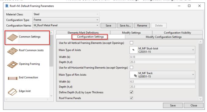
**Use for all Framing Elements (except Openings)** – if ON, then the selected Joist and Rim Joist families will be used for other framing elements, like connections, bridgings, noggings, etc. without an option to change it to a custom family.
