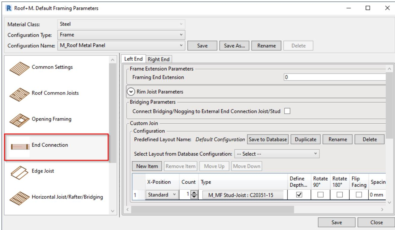
**Roof+** supports various types of end connections.
