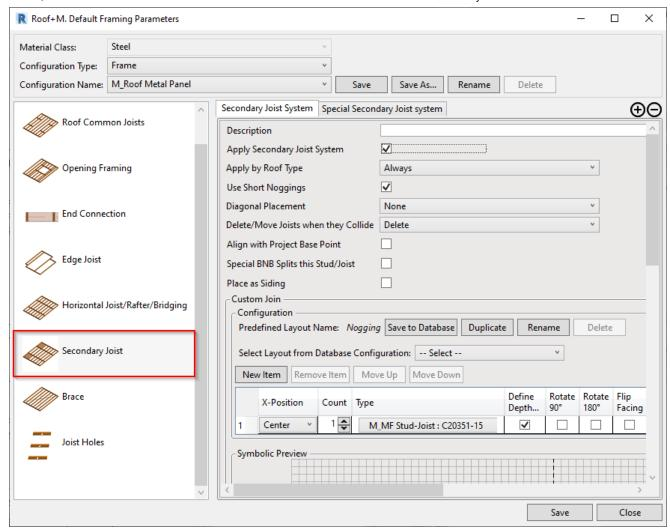
**Secondary Joist** – settings to add secondary joist system. It has the same settings as **Horizontal Joist/Rafter/Bridging**.
