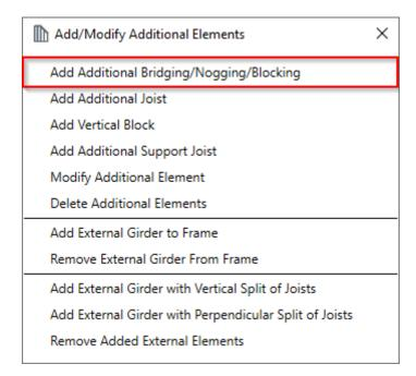
**Add Additional Bridging/Nogging/Blocking** – adds additional bridging/nogging/blocking between two selected joists with predefined settings.
