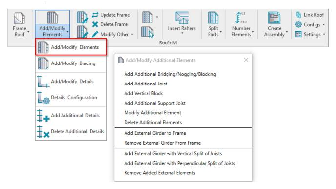
Add/Modify Elements – features for adding/modifying additional joists, support joists, bridging/nogging elements, etc.
