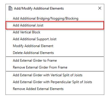
Add Additional Joist – adds additional joist into selected frame with predefined settings.
