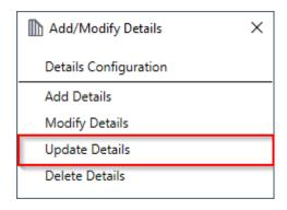
Update Details – updates details if any changes were made to roof, e.g. opening was moved, roof was extended, etc.
