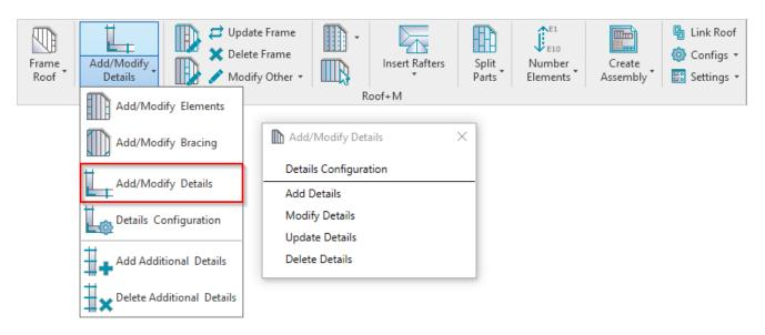
**Add/Modify Details** – for placing details in the frame. It is recommended to use these functions at the end of the framing process.
