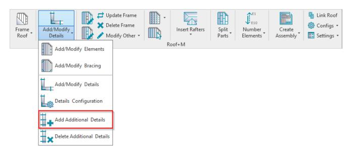
Add Additional Details – adds additional details by predefined rules to selected joist or rim joist.
