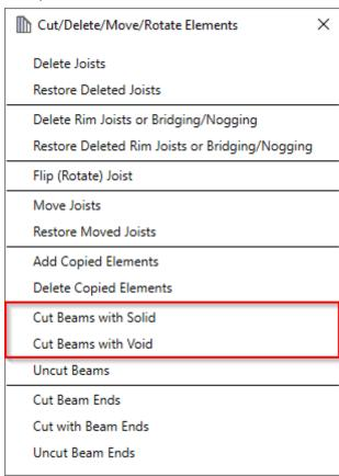
Cut Beams with Solid/Void - cuts beams that intersect with another beam (solid/void).
