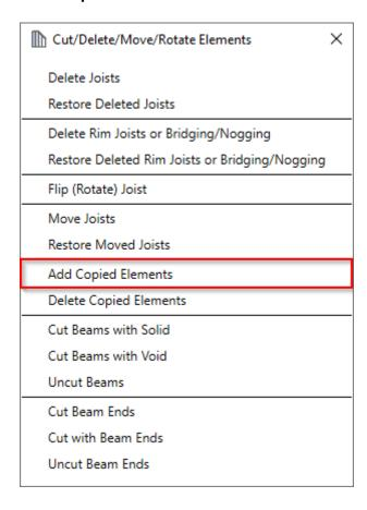
**Add Copied Elements** – adds copied elements to the existing frame system for later scheduling and inclusion in shop drawings.
