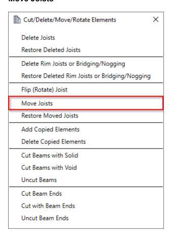
**Move Joists** – moves selected joist(s) to the left or right by predefined distance.
