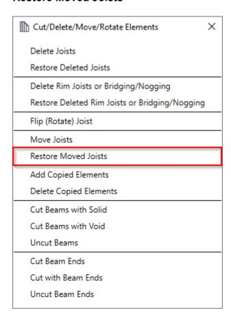
**Restore Moved Joists** – restores moved joists in selected frame to original position.
