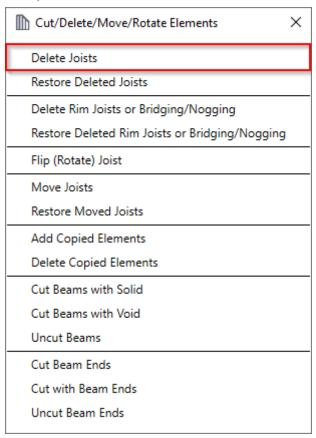
**Delete Joists –** deletes selected joists from the frame.
