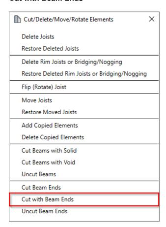
Cut with Beam Ends – cuts connected beam with selected beam ends.
