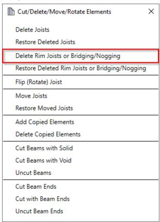
**Delete Rim Joists or Bridging/Nogging** – deletes selected plates or bridging/nogging which were inserted before. You can't delete it manually, because using updating functions the element will be restored.
