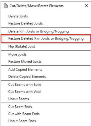
Restore deleted Rim Joists or Bridging/Nogging – restores deleted joists in selected frame.
