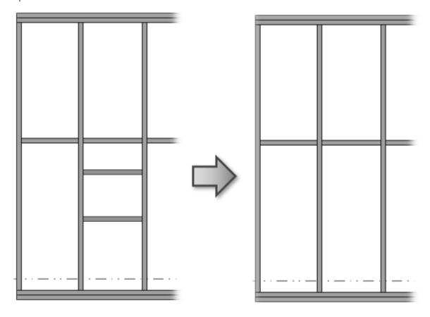
**Cut Beams with Solid/Void**
