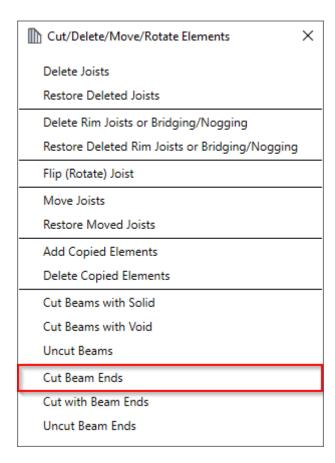
Cut Beam Ends – cuts selected beam ends that connect with another beam.
