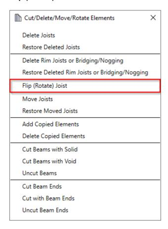
Flip (Rotate) Joist - flips or rotates selected joist.
