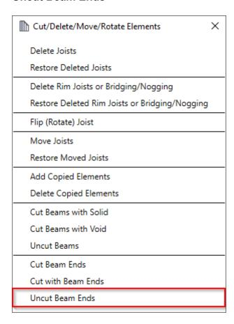
**Uncut Beam Ends –** uncuts beam ends that connect with other beams.
