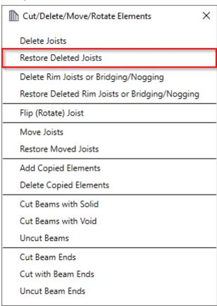
Restore Deleted Joists – restores deleted joists in selected frame.
