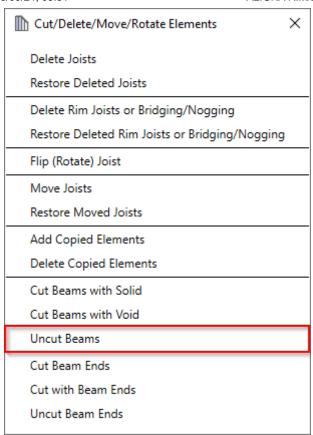
Uncut Beams – uncuts beams that intersect with another beam (solid/void).
