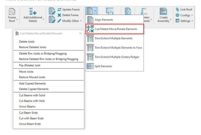
Cut/Delete/Move/Rotate Elements - features for deleting, moving, flipping joists, cutting beams, etc.
