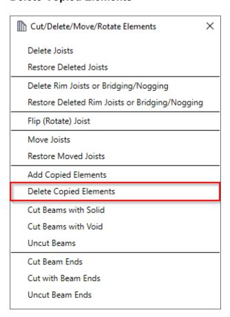
**Delete Copied Elements –** deletes elements that were copied manually and added to the existing frame system with **Add Copied Element**.
