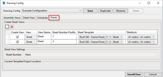
**Roof+M** creates sheets in the roof assembly using predefined settings.
