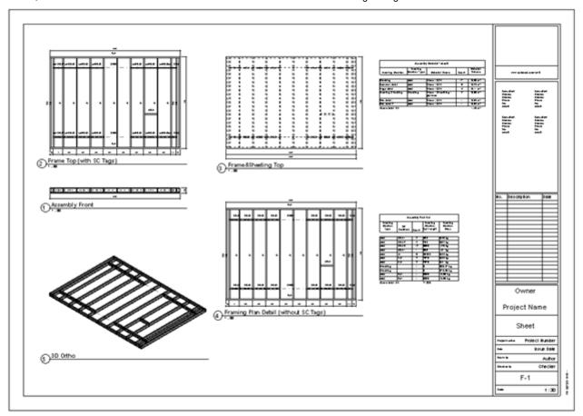
Create first assembly  $\rightarrow$  add views to the sheet manually  $\rightarrow$  open **Drawing Configuration**  $\rightarrow$  **Sheets**  $\rightarrow$  select a sheet to be a template for other roofs.
