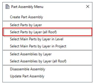
Select Parts by Layer (all Roof) - selects all framed parts in the roof.
