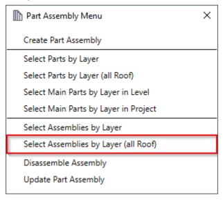
**Select Assemblies by Layer (all Roof)** – selects all part assemblies from the same roof. You just need to select one assembly and the others will automatically be selected.
