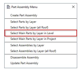
Select Main Parts by Layer in Level - selects main parts in roof frames of the same type in the same level.
