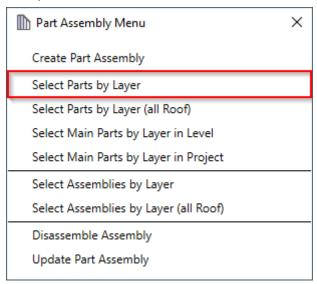
Select Parts by Layer - selects main parts in the framed roof.
