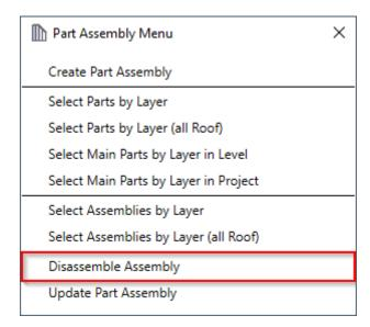
**Disassemble Assembly** – removes the assembly relationship between elements in the selected assembly and all associated views.
