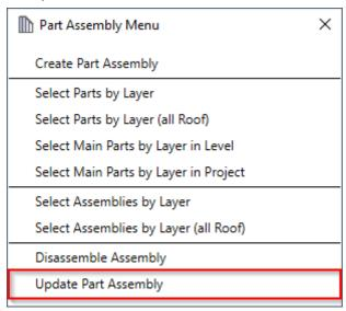
**Update Part Assembly –** updates the selected part assembly if any changes were made to the parts or to the **Drawing Configuration**.
