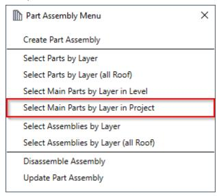
Select Main Parts by Layer in Project - selects main parts in roof frames of the same type in the whole project.
