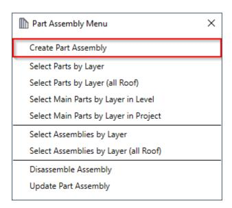
**Create Part Assembly** – makes shop drawings for selected framed parts. Select any frame of the roof and click Create Part Assembly. The software will create shop drawings according to predefined configurations. You can find shop drawings in Project Browser under Assemblies.
