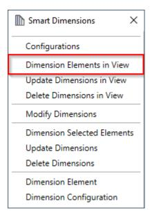
**Dimension Elements in View** – inserts dimensions for elements in the current view according to predefined configurations.
