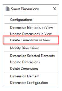
Delete Dimensions in View – deletes all dimensions that were added with Smart Dimensions from the current view.
