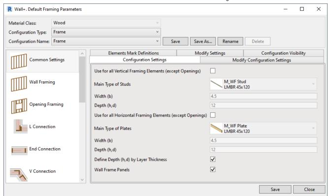
**Framing Configuration** – defines all framing settings. It allows user to configure and save settings for all sorts of frames – **Main Wall Frames**, **Secondary Frames**, **Vertical** and **Horizontal Nailers**, **Vertical** and **Horizontal Sidings**, **Wood Logs**. It is very a versatile tool with thousands of possibilities.
