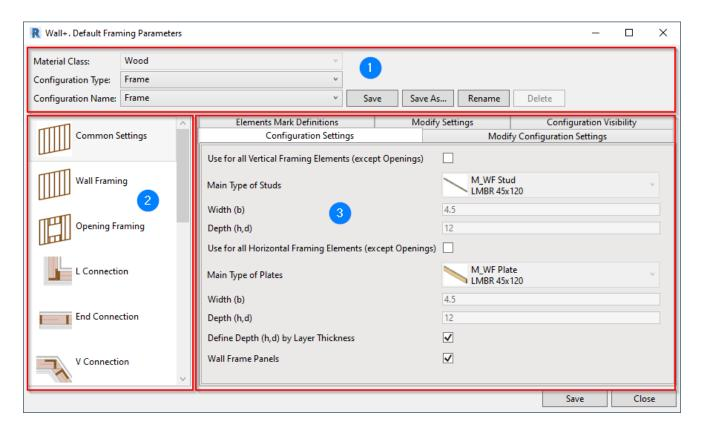
The Framing Configuration dialog is divided into three main parts: Top (1), Left (2) and Right (3). In the Top part, choose the Configuration Type that you want to use and Configuration Name that you want to modify.
