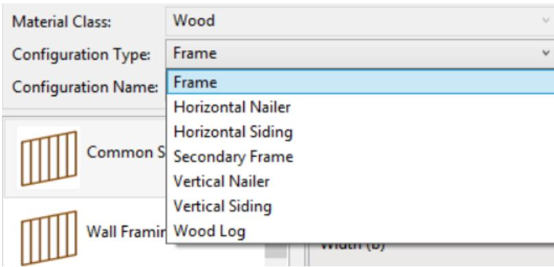
**Configuration Name** – configuration with all framing settings. You can use sample or create new configurations. Also, you can rename or delete the existing configurations.
