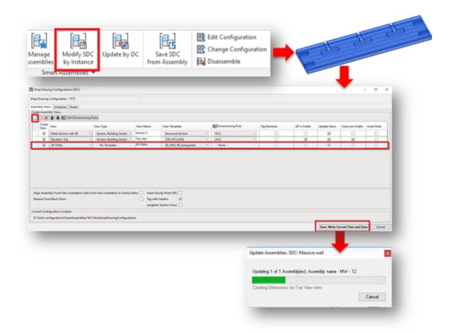
After you change these individual configurations, the assembly will be updated according to the changes you made, and in the SDC Instance parameter you will see that the name of configuration has changed. It now has an added prefix – **Instance\_**.
