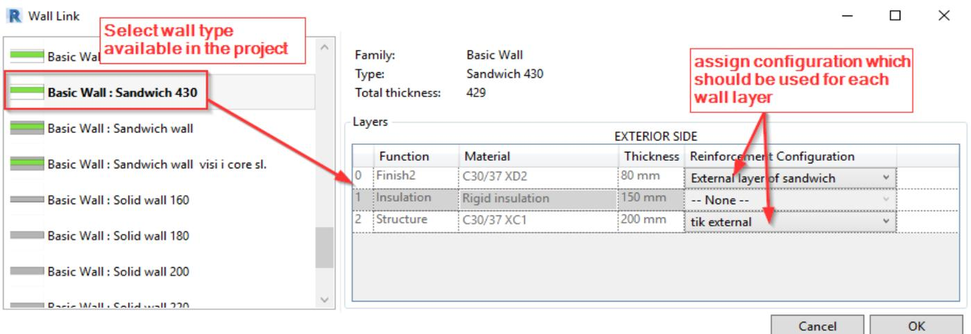
Now you can use the Create Rebar command for this wall type which already has configurations assigned through the Wall Link.
