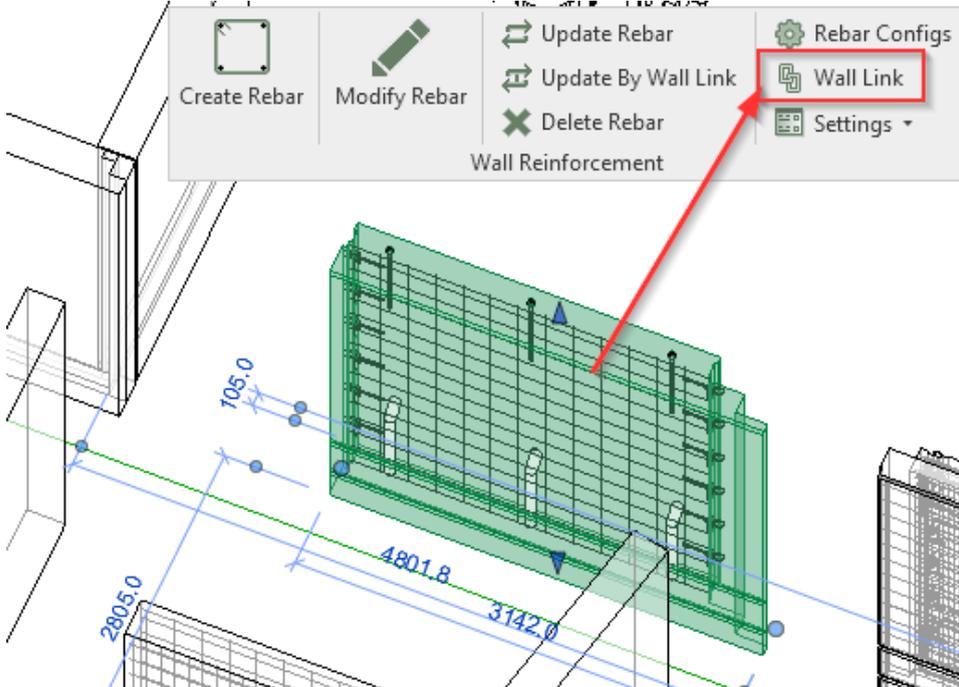
3. In the following dialog window assign configuration for each layer which should be reinforced.
