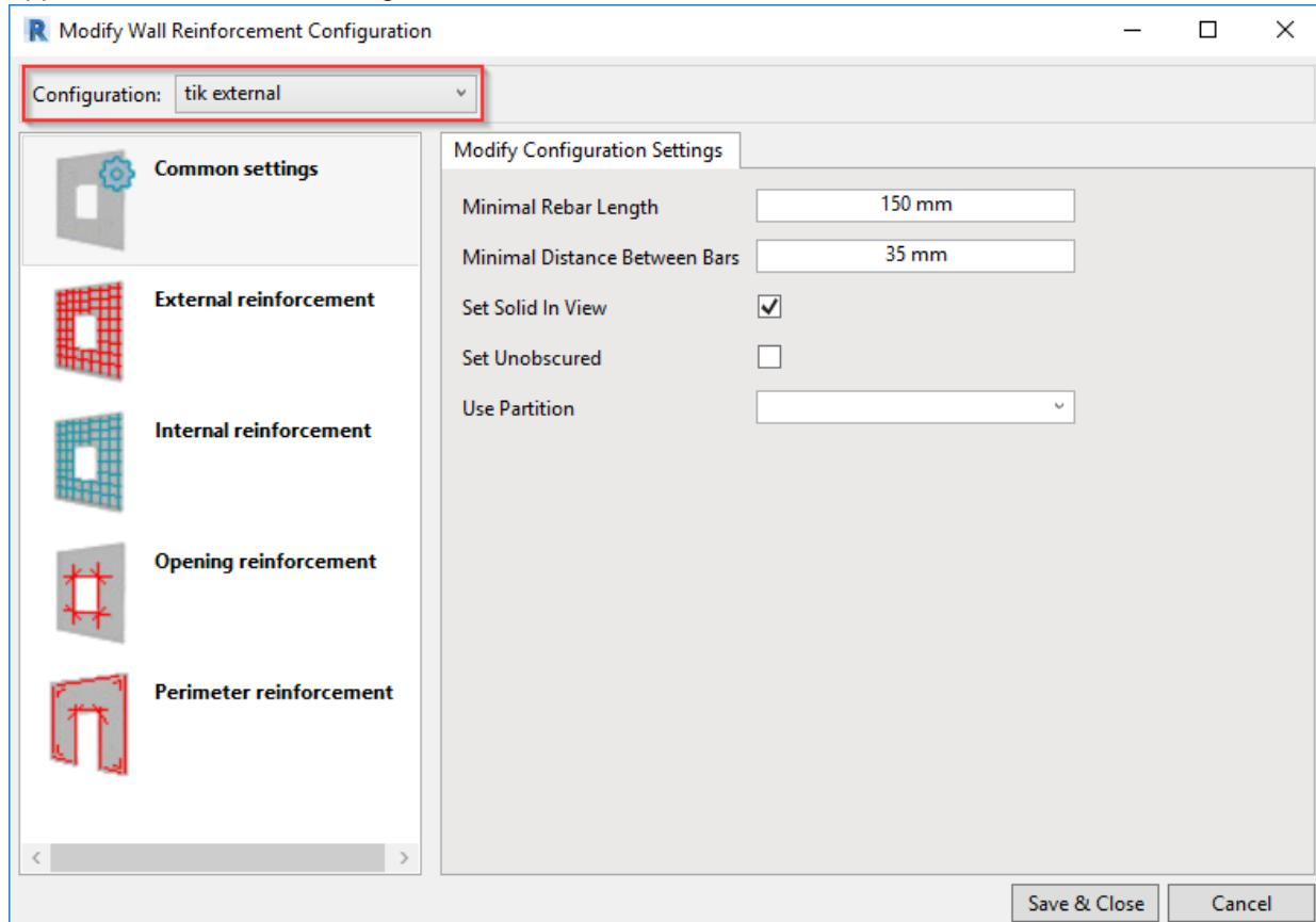
3. Make changes in configuration window – add other rebar, switch off selected rebar, change rebar type, step, hooks, or other settings – and finish with Save & Close.
