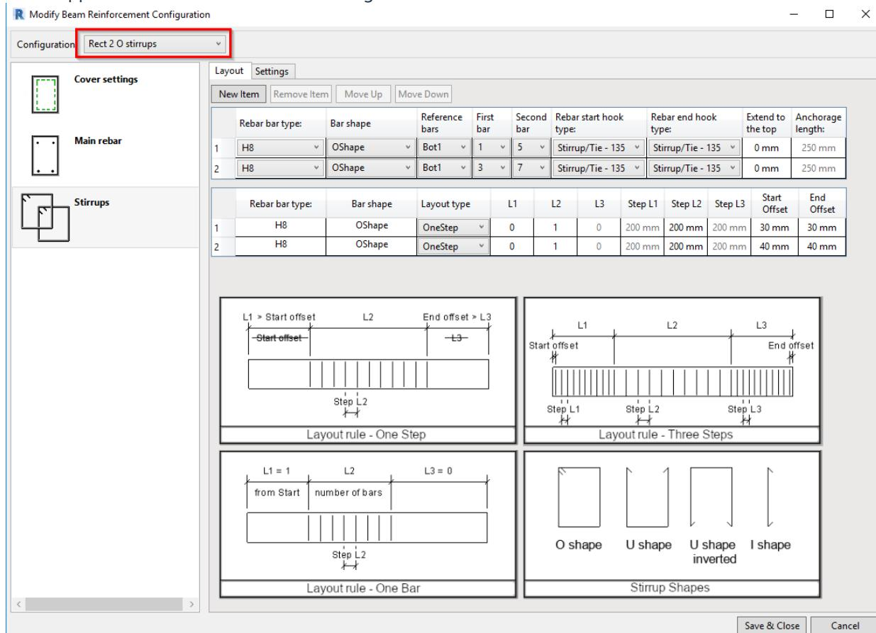
3. Make desired changes in configuration window – add rebar, switch off selected rebar, change rebar type, step, hooks, or other settings – and finish with Save & Close.
