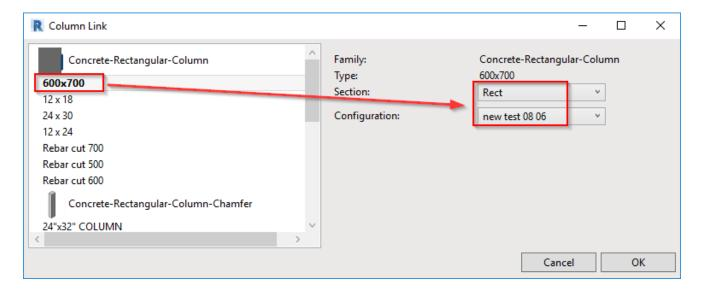
4. Select Structural Column(s) with the Type used in Column Link, and use **Create Rebar** command. It will read which reinforcement configuration should be used from the Column Link and will then create rebar.
