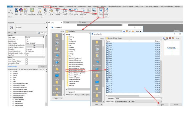
2. Prepare **Rebar Configuration** for selected column section.
