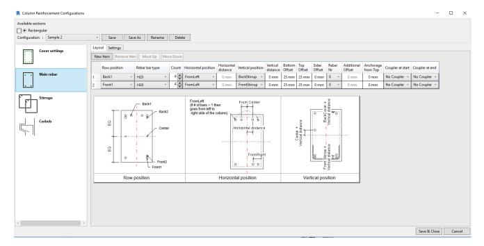
3. Assign configurations to Structural Column Types by using **Column Link** (https://agacad.freshdesk.com/en/support/solutions/articles/44001982871-cr-column-link).
