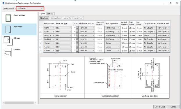
3. Make desired changes in configuration window – add rebar, switch off selected rebar, change rebar type, step, hooks, or other settings – and finish with Save & Close.
