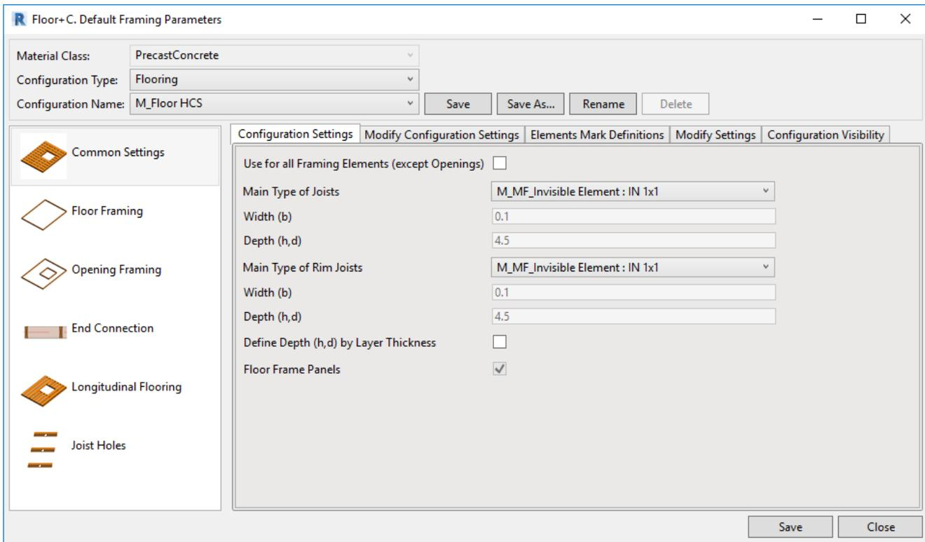
Floor+C tool was created based on Floor+M tool (for light gauge steel) platform, so it is usually not necessary to adjust some of the settings for precast concrete slabs.
