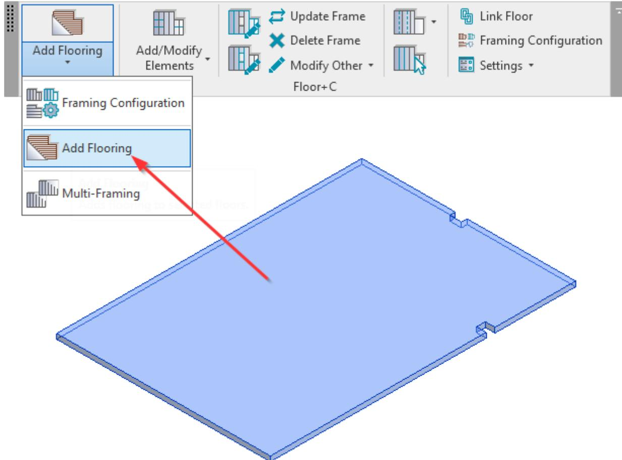
Layout of Structural Framing will be created based on configurations:
