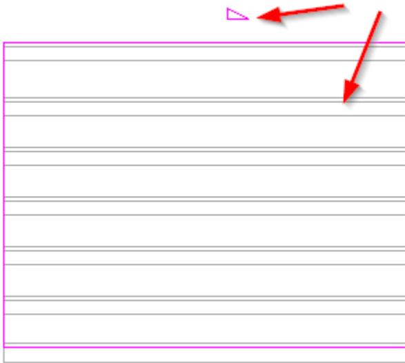
*If there is Slope Arrow used in the roof creation then the joists will be perpendicular to it:*
