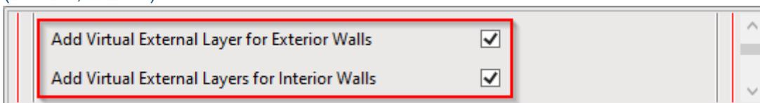
**Add Virtual External Layer for Exterior/Interior Walls** – adds virtual layers for exterior/interior walls that are mostly used for siding finishing/decorations.
