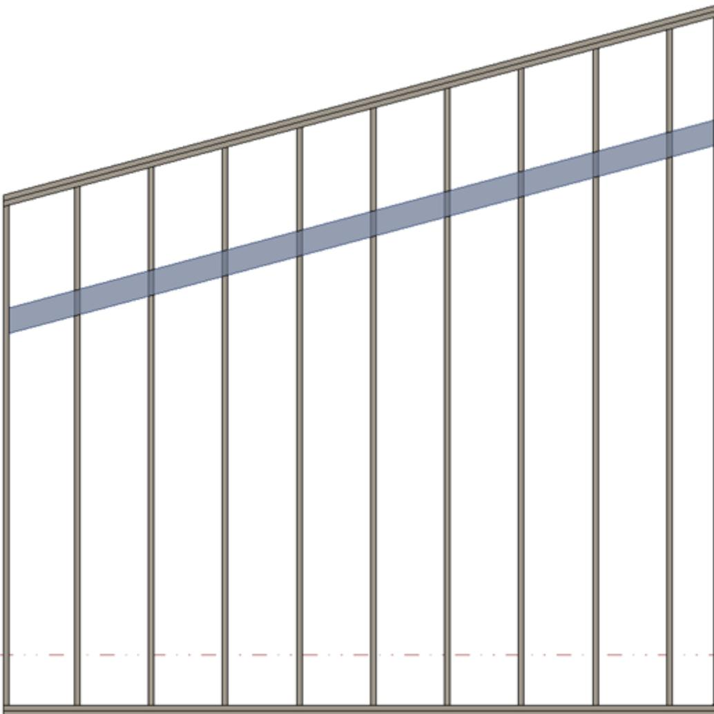
*Example: Blocking is placed parallel to top sloped rim joist:*
